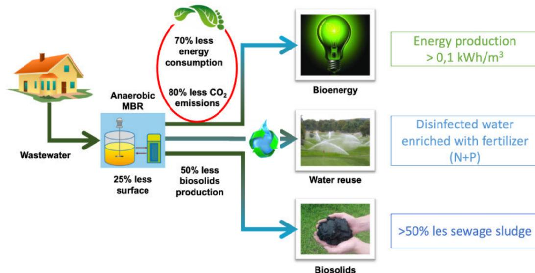
Figure 2: Anaerobic Treatment to Convert Wastewater to Methane - Graphic by Aqualia
