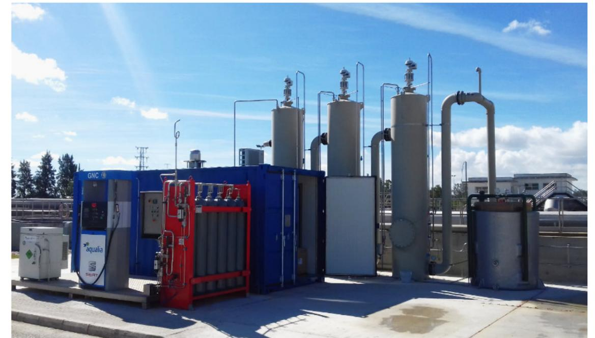
*Biomethane filling station and biogas upgrading (ABAD Bioenergy®) installed in Jerez WWTP (Spain) – SMART GREEN GAS PROJECT*
