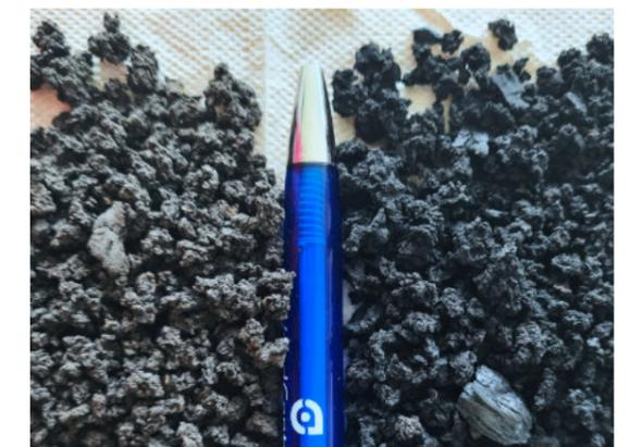
Figure 6: Biochar from pyrolysis and Biosolids 90% Dry Matter - Photo by Ivan Volund
