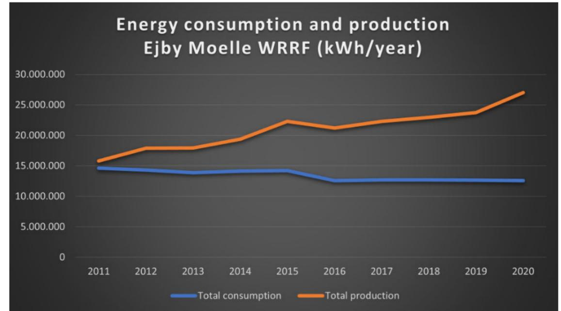
Figure 1: Energy consumption and production at Ejby Moelle Water Resource Recovery Facility - Graph by Ivan Vølund
